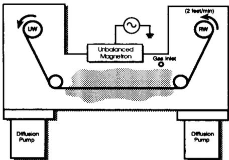
(FLEX-1) 0.66 meter Web Width Prototype Web Coater
